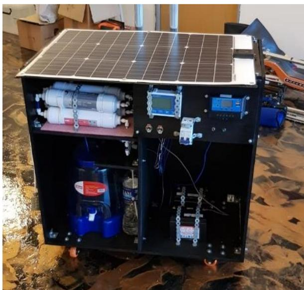
*Prototype of the portable solar-powered filtration unit that Kunal presented as his project for a bachelor programme’s module in 2019. (Photo: Kunal Ghanisham)*
